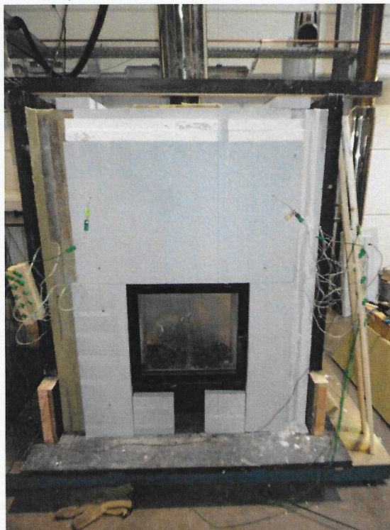
Map. 5 Test installation of the first test - Installation is heated dry (still with open convection air channels)
